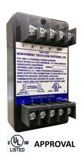
**Northwest Tech-Con Systems** <u>ISB</u> has been created as a 4-channel Intrinsically Safe Barrier. The barrier provides intrinsically safe outputs for connection to level floats, non-inductive resistive devices, switches, RTD's, input of PLC and thermocouples or a variety of sensors in Class 1, Group D locations.
