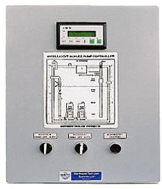
Northwest Tech-Con System's HPC has been recently developed for water and fuel applications. The controller utilizes an embedded microcomputer and a hydrostatic floatless liquid level transducer in the pump chamber to continuously monitor liquid levels, and control the operation of pump(s). Users can change settings on the control panel at the data terminal to define the level of stop / start / override / lead / lag / alternate / alarm status.
