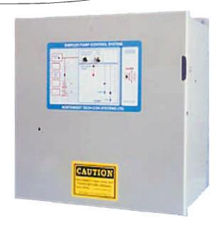
Northwest Tech-Con Systems I-SCP Intrinsically Safe Simplex Controller is specifically designed and approved for Class 1, Division 1, Group D, and Hazardous Operation. The Intrinsic Barrier generates extreme low voltage in the float circuit, which will prevent hazardous materials from igniting. For more information see section ISB and SCP.
