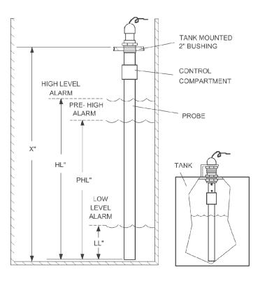
PROBE MODEL: HPP - X" TANK DEPTH IN INCHES
